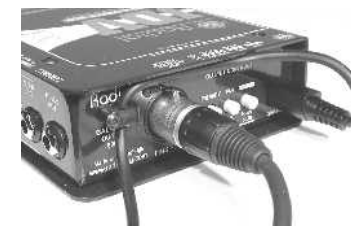
The JDV's strain relief in action.
